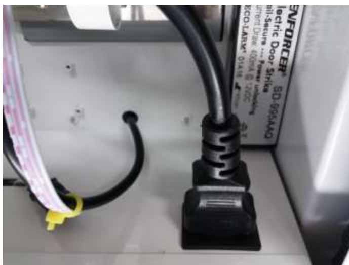
Standard cable with fixed IEC C14 Type F plug
