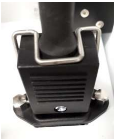
Alternative IEC C14 Type F plug and Type E socket with retention clip
